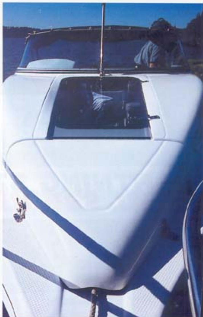
Anchoring is done from either the walkround deck or through the big side opening hatch. The anchor locker open to the side, but has a niche moulded in for the anchor warp.
