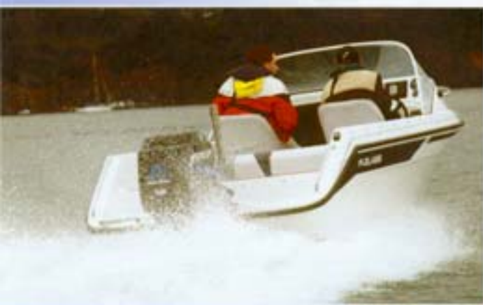
The Fi-Glass Senator is an easily driven hull with the single planning strake doing its job well
