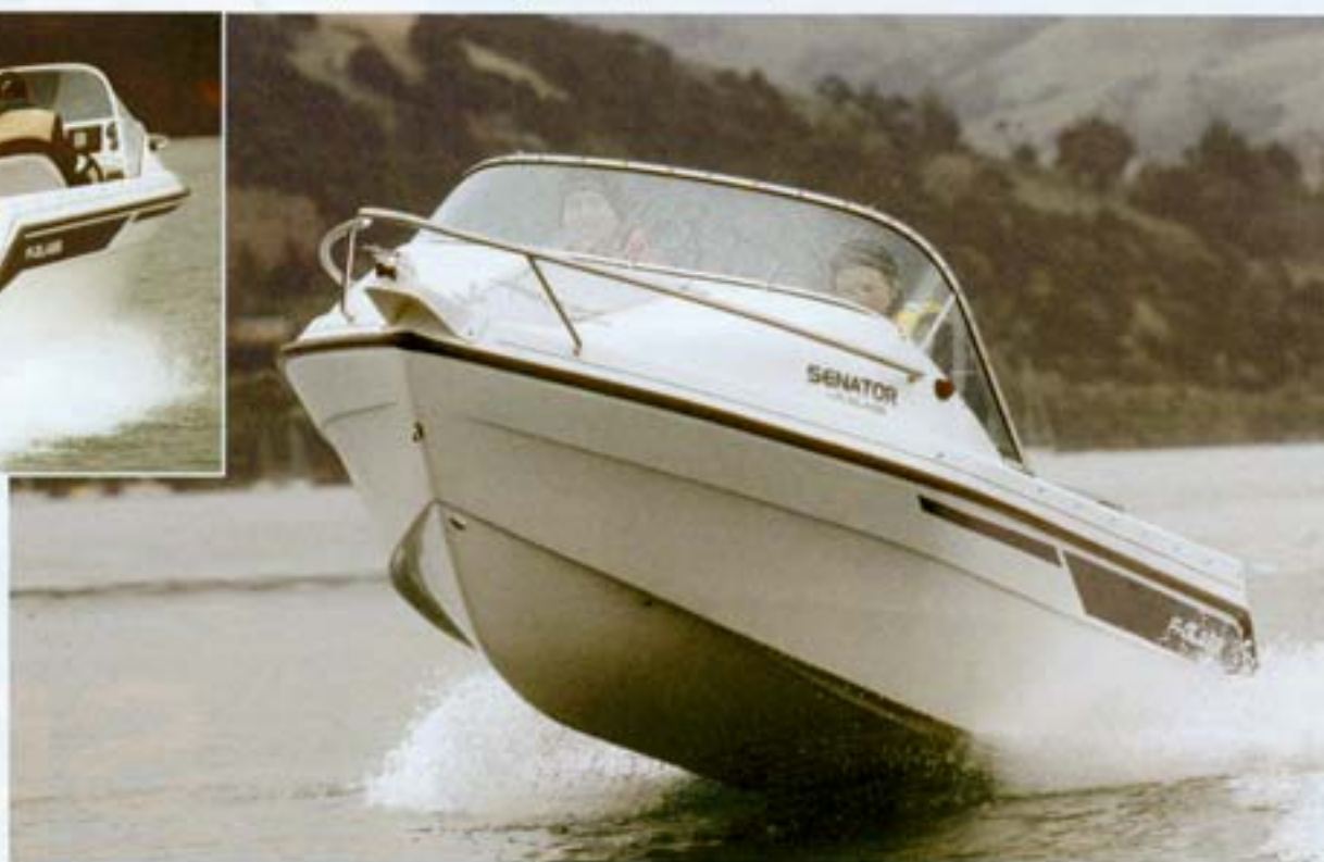
The Fi-Glass Senator is an easily driven hull with the single planning strake doing its job well
